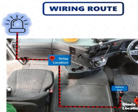
Gambar 2. Wiring Route Advance Safety Belt
