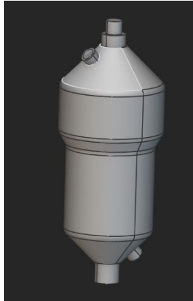
Figure 2 oil cooler design
