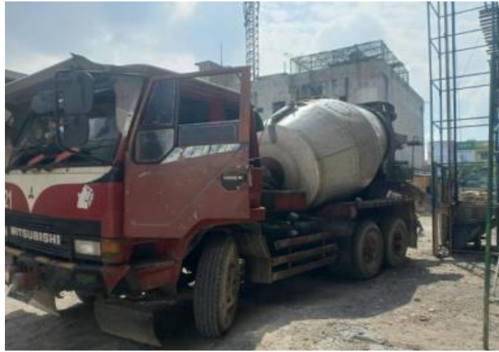
Gambar 2. Truck Ready Mix
