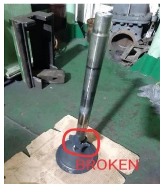
Gambar 3. Valve spindle rusak Sumber: MV. PAN IVY.
