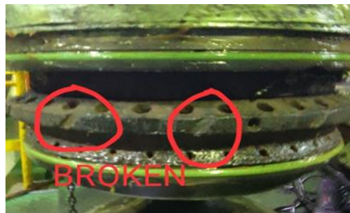
Gambar 2. Seat valve rusak Sumber: MV. PAN IVY.
