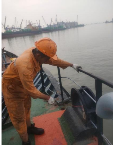
Gambar 7. Pengecatan Marine Panama Chock
