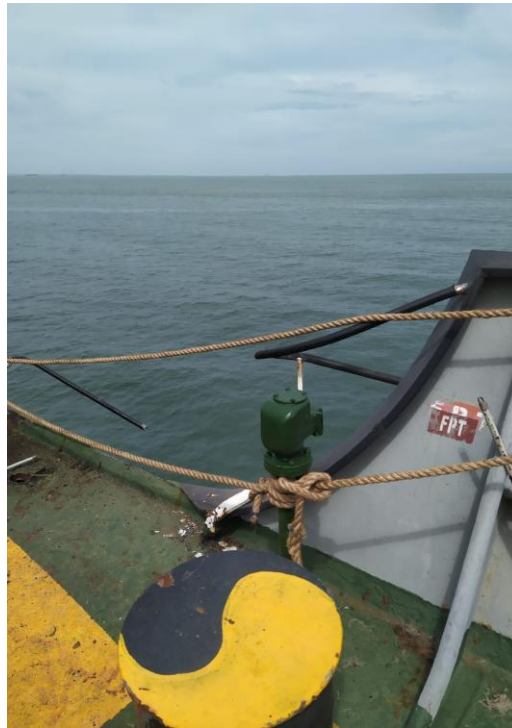
Gambar 3. Marine Panama Chock dikapal MV. XYZ Terlepas
