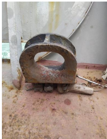
Gambar 2. Marine Panama Chock dikapal MV. XYZ Berkarat
