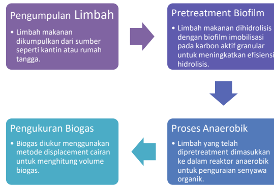
Gambar 3. Diagram Proses Pengolahan Limbah Berbasis Biogas [34]
