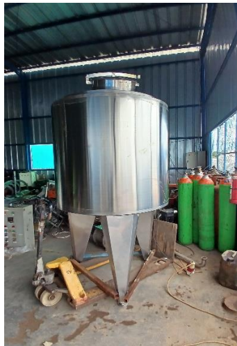
Gambar 1. Mesin Heating Tank
