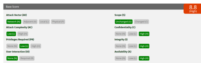
Gambar 11. CVSS ( Broken access control )
