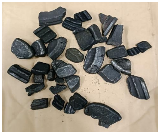
Gambar 14. Material Pecahan Exhaust Valve
